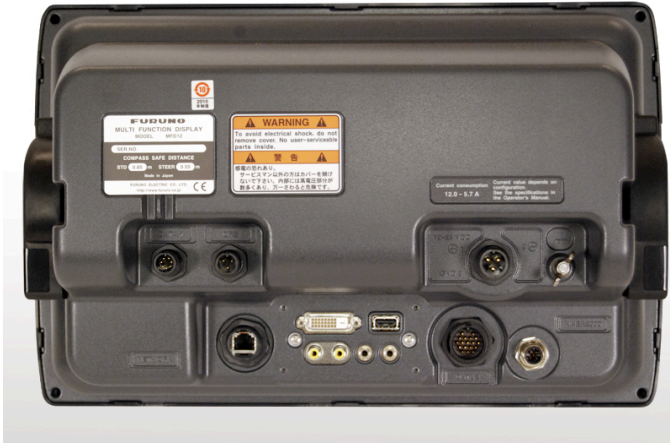
Today's modern MFDs feature numerous inputs/outputs for connections and networking
